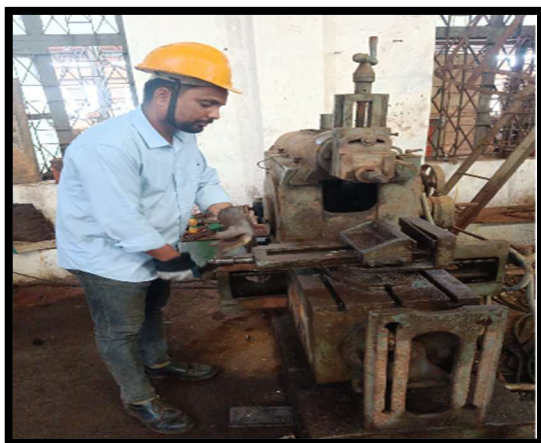
SHAPER MACHINE & SURFACE GRINDER FOR SAMPLE PREPARATION
